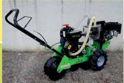
Precision single-seed planting system which allows to proceed seed by seed, independently from type and size. Unique on the world market: no friction, smooth and unalterable; the seeds are held on an adjustable groove, which at the right moment detaches the seed with a soft blow. The seed container and protections are made of see-through material, so as to allow users to check whether it is working properly.
